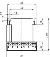
Mounting bracket set for 35 mm rail acc. EN 60715: Article No. 1802911
