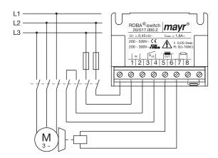
DC-side switching means short brake engagement times (e.g. for EMERGENCY STOP operation); but louder switching noises will occur.
