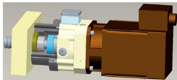
Lower Illustration: the same design; but this time with an additional brake. The ROBA®-topstop® single circuit brake with integrated ROBA®-ES shaft coupling is especially conceived for mounting on a ball screw spindle. The coupling housing is much shorter, meaning that the total construction increases only minimally in length. The shaft coupling becomes a brake component.
