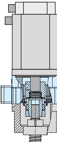
Brake system with integrated, plug-in shaft coupling. Separate coupling and coupling housing are no longer necessary.
