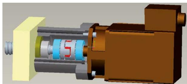
Upper Illustration: a typical servomotor attachment with a shaft coupling on an axis with a ball screw drive. The coupling housing ensures the necessary distance between machine and servomotor.
